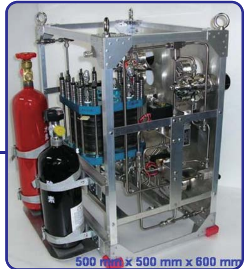
100W-Class Fuel Cell System to Mount to Observation Balloon (Japan Aerospace Exploration Agency)
