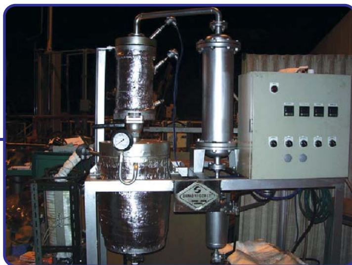
Experimental Apparatus for Small-Scale Hydrogen Production from Waste Plastics Using the Catalytic Steam Reforming Process (Tokyo Institute of Technology)
